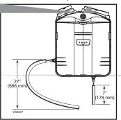
Cut 2 sections of plastic tubing; one 7" (178 mm) long and one 27" (686 mm) long, and attach them to each drain fitting as shown.
